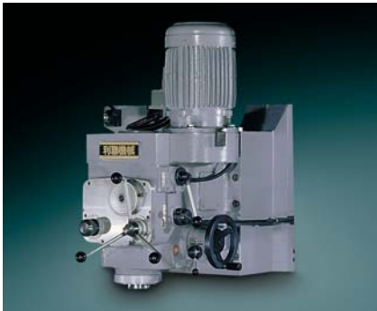
OX-1 Gear head (NT40/16 Steps/70-3540rpm)
