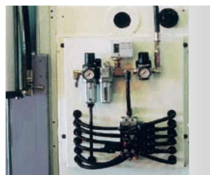
Pneumatic parts in one plate easy to inspect and maintain.
